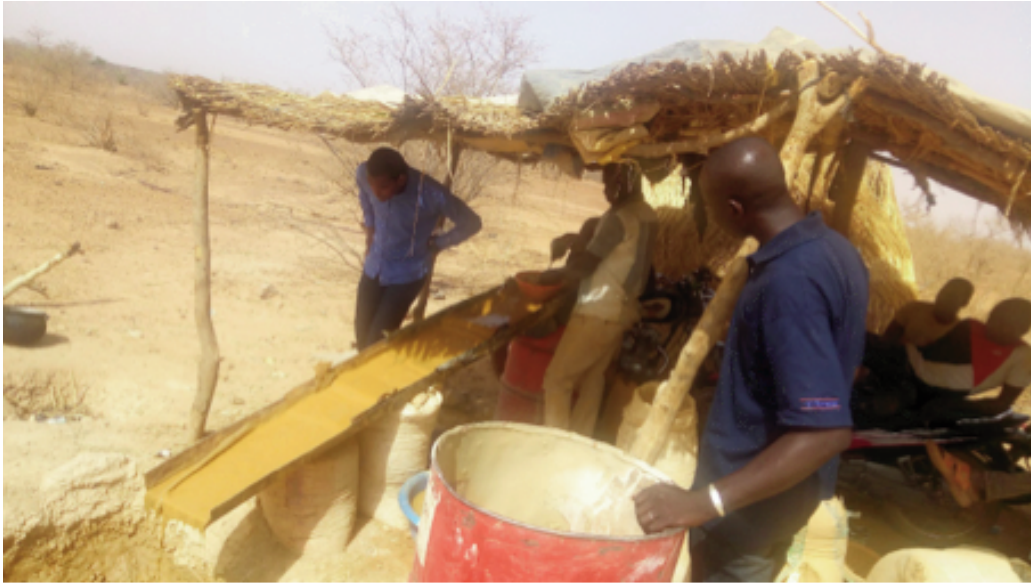
Illustration 2: ore powder washing station.
